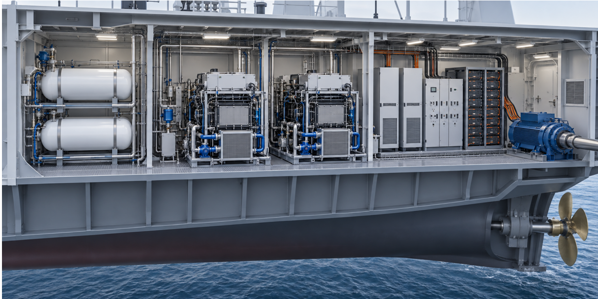
Figure 5.1: Conceptual PEM fuel-cell machinery room with redundant trains, power electronics and thermal management.
